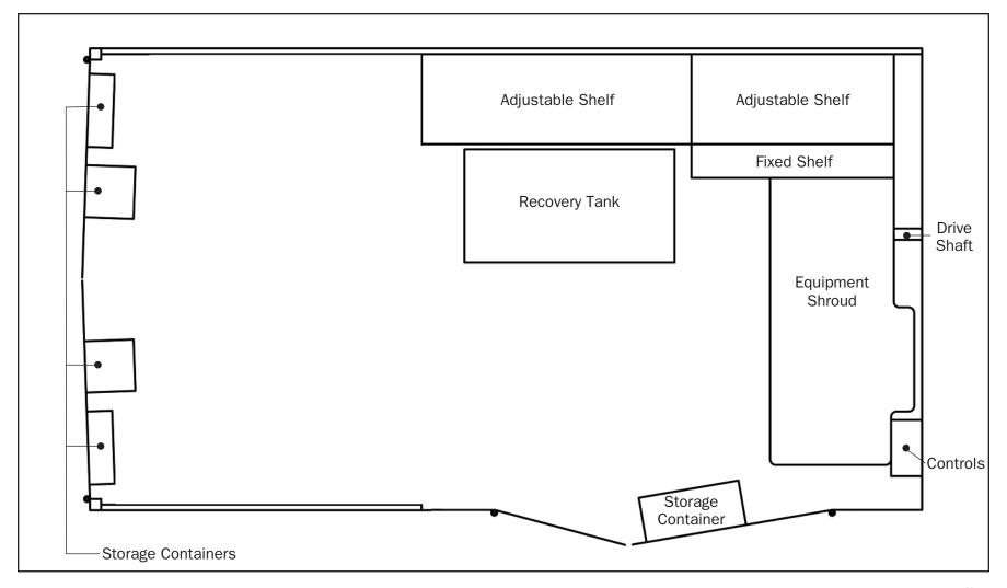
Floor plan is to exact scale in a 12' long cargo body.
