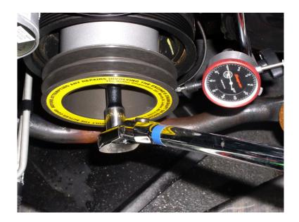
6. Continue rotating engine crankshaft clockwise until the lowest point on the pulley is shown on the dial indicator.
