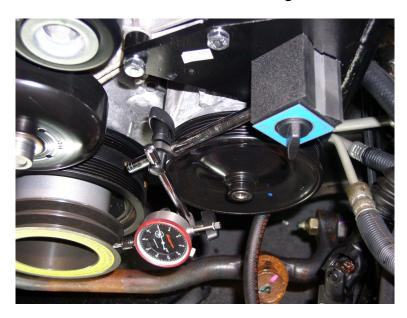
2a. 2021 and newer vehicles with 4.3L V6 & 6.6L V8 engines must use the dial indicator mounting plate available to rent in our crankshaft drill kits and dial indicator kits.(Suggested dial indicator mounting position shown below.)
